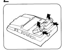
Rotate the stand ½ turn so that the arrow on the stand shows UP for WALL.
