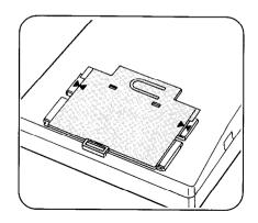
Push the two shaded portions slightly and insert the edges of the holder under the slide rails and then slide down toward arrow "A".
